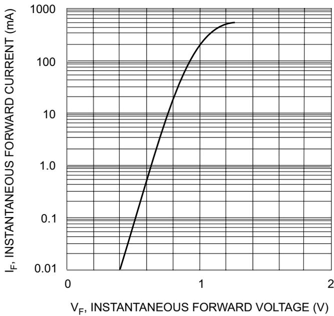
Fig. 1 Forward Characteristics
